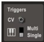
The **Trigger CV** input is used to retrigger Shape based on its **Run Mode**. See the **Trigger & Run Mode** Section.
